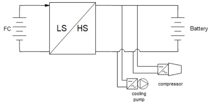
Figure 8: General schematic of the HV system.
