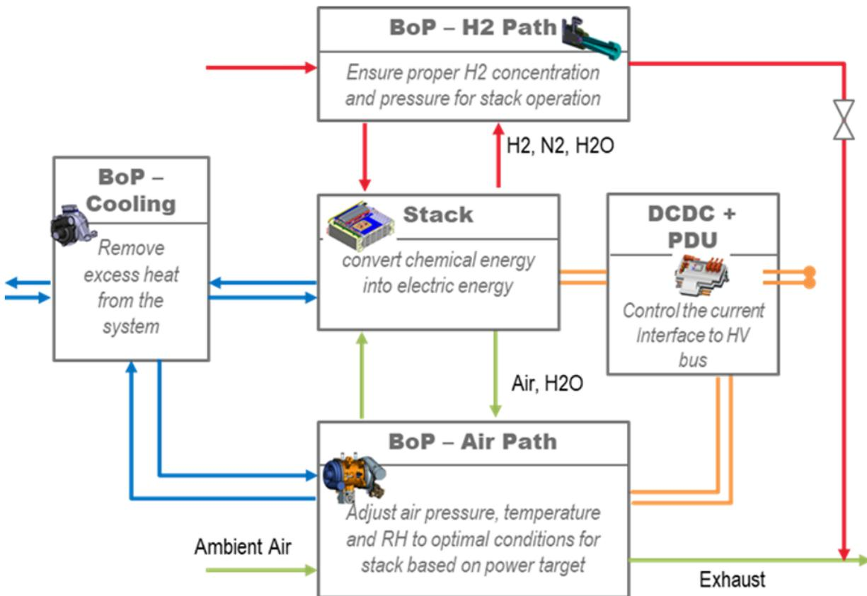
Figure 7: Overview Fuel Cell System Architecture.
