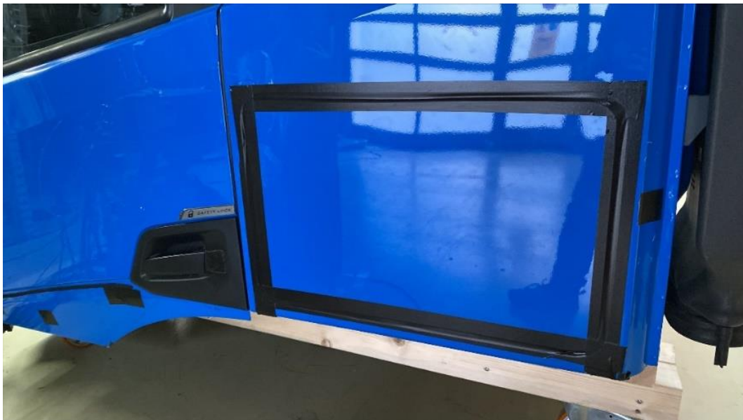
Figure 6: Sealed side compartment doors, to simulate improved rubber sealings.
