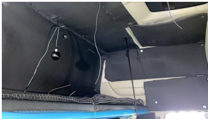
Figure 1: Insulation of overhead area.
