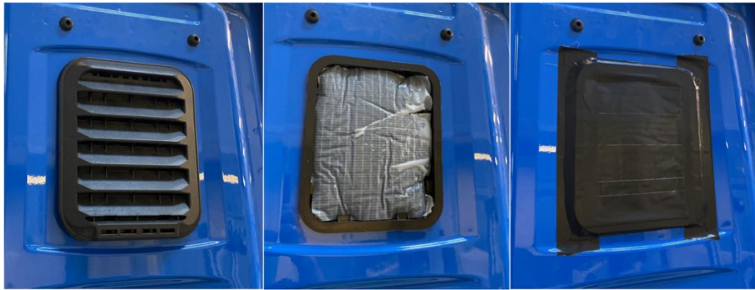
Figure 5: Insulating and sealing main cabin opening.
