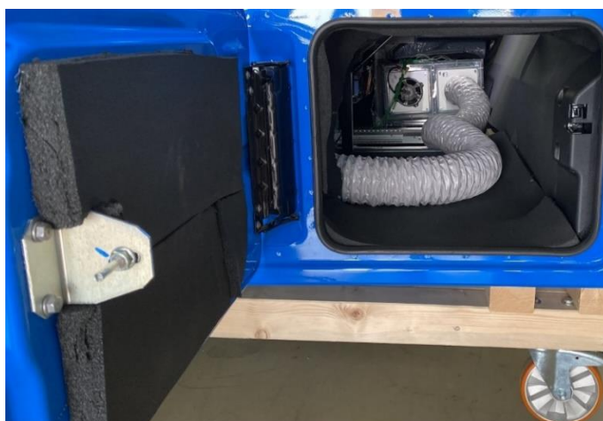
Figure 2: Insulation of compartments.
