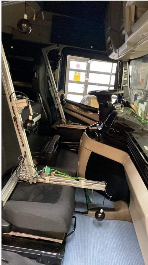
Figure 3: Floor insulation and removed dashboard piece (right side of the cabin).
